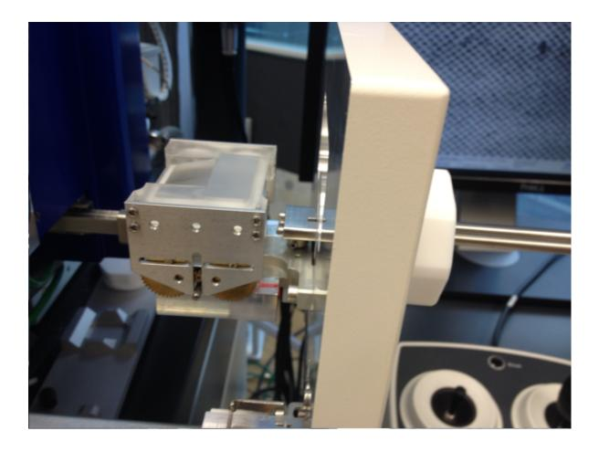
Sample Transfer Shuttle for ZEISS FE-SEMs and SEM/AFM hybrid systems Protect your sample from air exposure
